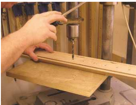
▲ Pic.14 Use a mortise gauge to mark the position of the shelf sockets centrally on the rear upright, then drill the holes
